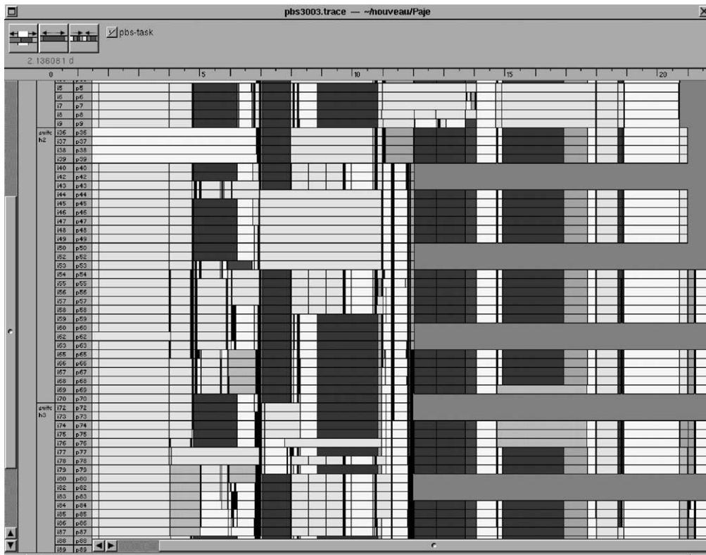
Fig. 8. Scheduling of jobs on a large-sized cluster. Each line represents a different processor of a 100 processors cluster. The three columns on the left identify interconnection switches, nodes and processors (there is a single processor per node in the example). Each color represents a different user reservation.
